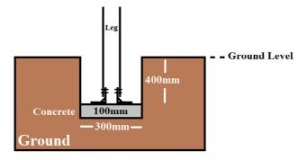
5. Once the canopy erecting has been completed, check the legs are level and back-fill the remainder of the hole.
