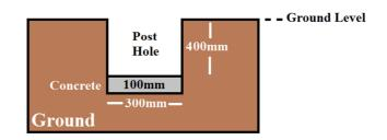
4. Once the feet have been fitted to the leg, stand the foot on the 100mm, hard foundation.
