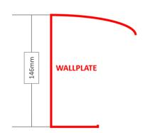
Example 1: 10 degree pitch, 3.5m projection – If you would like your gutter underside to be 2100mm then your wallplate height will be: 2,100+624 = 2,724mm
